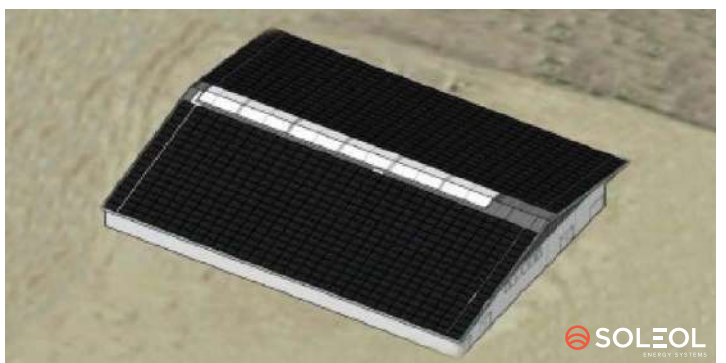
Project in Carrouge VD Panels 948 – Area 1,779 m 2 – Power 370 kW
